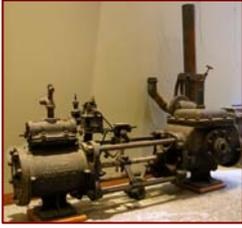
Now located in the lobby of Building 59, this single-cylinder **Burnham Simplex Pump (60-1-6)** was originally located in Building 60, the fire Pump House, to pump alcohol to and from railway cars stopped just south of the building. It also pumped antifreeze back and forth between tank cars and the Cannery scale tank loft. Patented in 1893, it probably dates from the 1890s.
