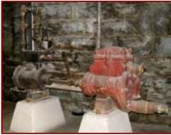
Now located in the Lobby of Building 5 in the Stone Distillery, this **Smart Turner Duplex Pump (56-1-3)** was originally located in Building 56 of the Pure Spirits complex to pump liquids during distilling operations. The red paint, however, may indicate that it was used to pump water for fire protection. The pump was manufactured in Hamilton, Ontario during the late nineteenth century.
