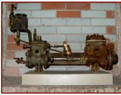
This little **Worthington Duplex Pump** is the smallest pump on display. Originally located in Building 47 and used to pump alcohol to the scale house in the Denaturing Building, the pump is now in a niche on the second floor of Building 5 in the Stone Distillery.
