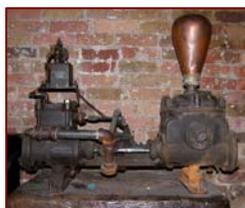
This **Worthington Duplex Pump (47-1-5)** was one of three pumps used in Building 47 during the denaturing process when chemicals were added to alcohol to render it unpalatable, untaxable, but still good for industrial alcohol purposes. It was probably created in the 1890s and is located near its original position.
